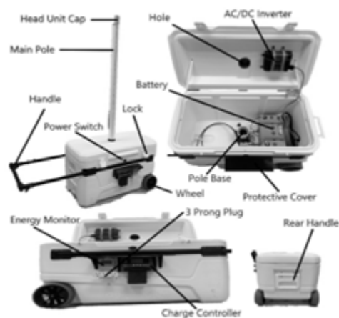
Figure 3: Final Solar Turtle Bottom Unit Assembly
