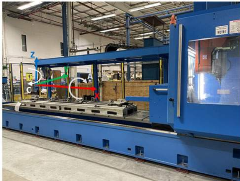
Figure 1. A picture of the Bavius CNC machining center. The machine coordinate system is superimposed on the picture. When the machine rotary axis A = 0^\circ , the spindle is vertical as shown.
