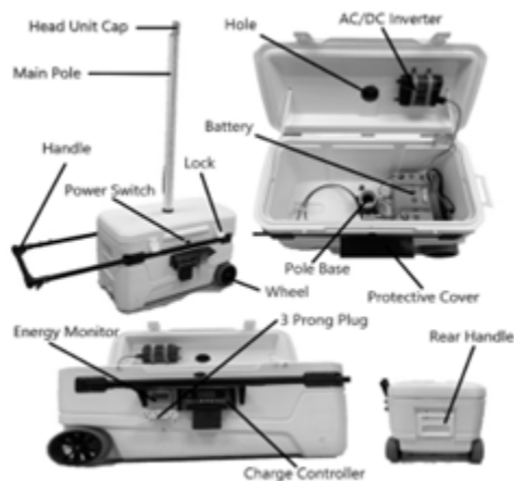
Figure 3: Final Solar Turtle Bottom Unit Assembly
