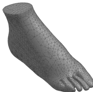
Figure 7. Finite Element Mesh Applied to Foot Geometry
