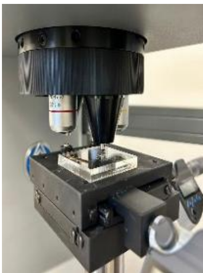
Figure 3. Vickers Hardness Tests for Polymer Laminates
